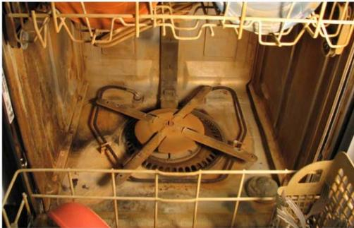
Top photo is of a dishwasher at the end of 30 days using soft water. Bottom photo is of a dishwasher at the end of 30 days using hard water (Battelle Study).
