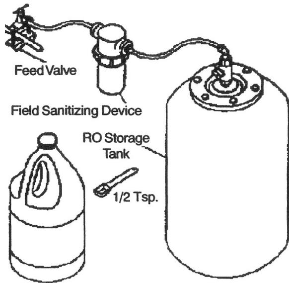
10. RO Holding Tank Cleaning Procedure: The procedure below uses chlorine as the disinfectant, but the same procedure could be adapted to other disinfectants by adjusting the dose accordingly.
